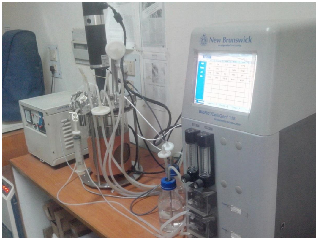
Fig. 3.2: 7.5 L fermenter (BioFlo/Celligen 115, New Brunswick, USA) Working volume (2.8-5.6 L)
