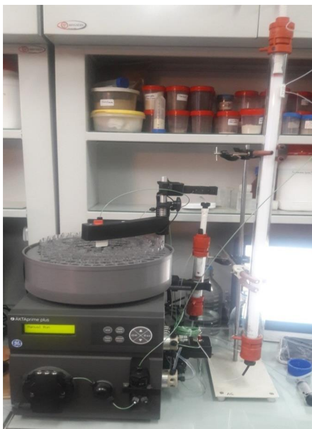
Fig. 3.5: Size-exclusion chromatography using Superdex-75pg column
