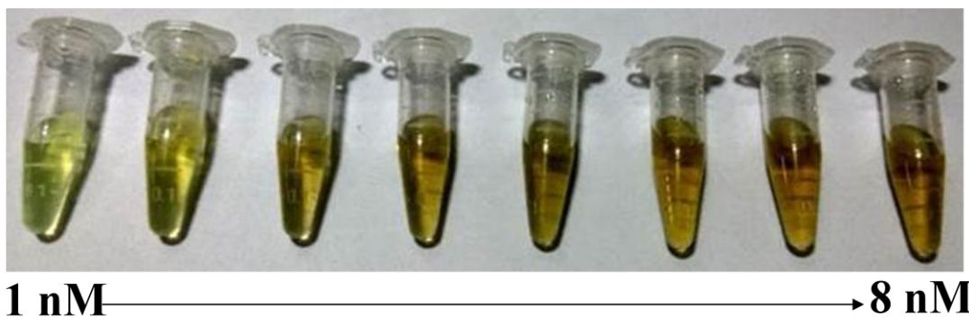
Figure 6.13 Photographs showing the color-change during colorimetric sensing of Picric acid.
