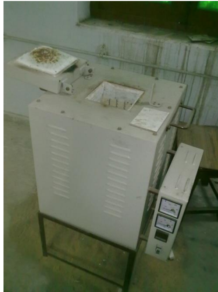
Figure 1. Stir casting Furnace
