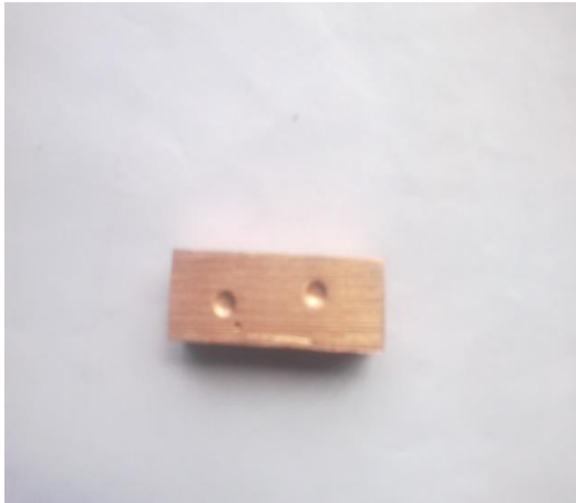
Figure 4(a). Hardness indentation of Cu-1wt%Cr-1%TiC Composite
