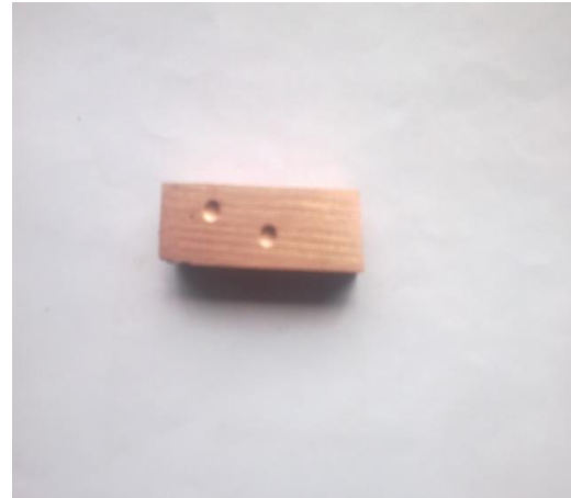
Figure 4(b). Hardness indentation of Cu-1wt%Cr-2%TiC Composite
