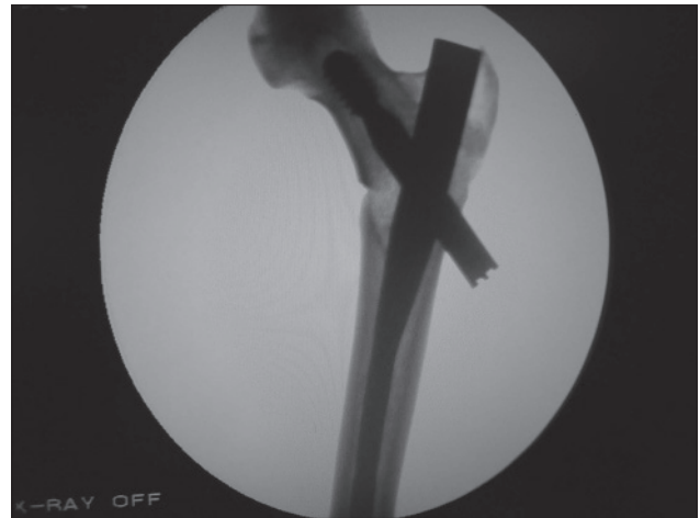
Figure 5: Fluoroscopic view showing this bone implant construct fixed with Gamma nail showed backing out of lag screw after 28,000 cycles. there is also displacement at the fracture site suggesting increased subsidence.this concludes Gamma nail is less stable in comparison to Gamma nail in unstable trochanteric fractures
