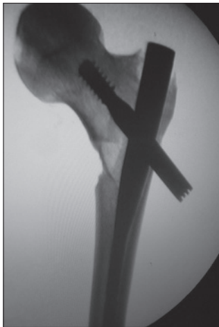
Figure 4: Fluoroscopic view showing this bone implant construct fixed with Gamma nail showed backing out of lag screw after 28,000 cycles. there is also displacement at the fracture site suggesting increased subsidence.this concludes Gamma nail is less stable in comparison to Gamma nail in unstable trochanteric fractures
