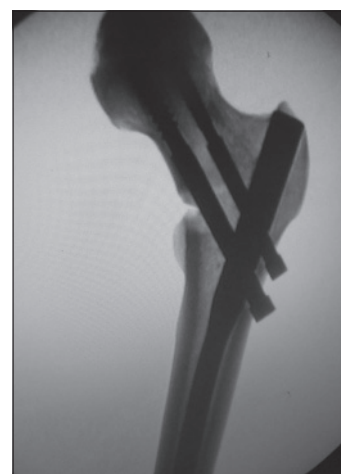
Figure 2: Fluoroscopic view showing specimen of cadaveric femur fixed with PFN and made unstable after creating posteromedial defect. This bone implant construct is mounted on MTS machine and tested with 200 kg load and 50,000 cycles
