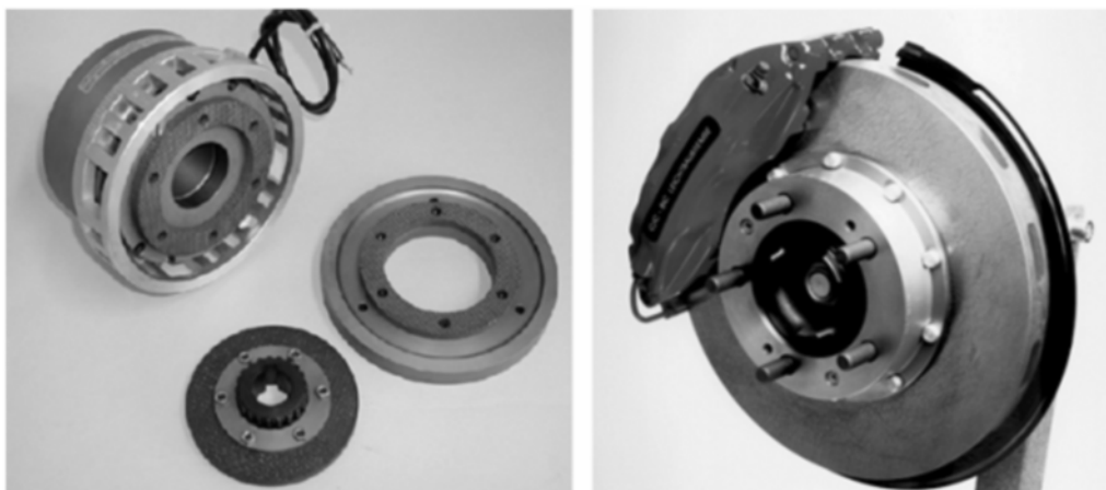
Fig. 1 Emergency braking system (left) and internally ventilated brake disc for passenger cars (right), made of C/C–SiC composites. Reproduced with permission from Ref. [37], © 2005 Kluwer Academic Publishers.
