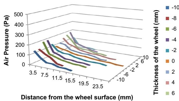
**Figure 15.** Variation of air pressure in radially outward direction and at various points along the thickness of cast iron wheel with scraper board.
