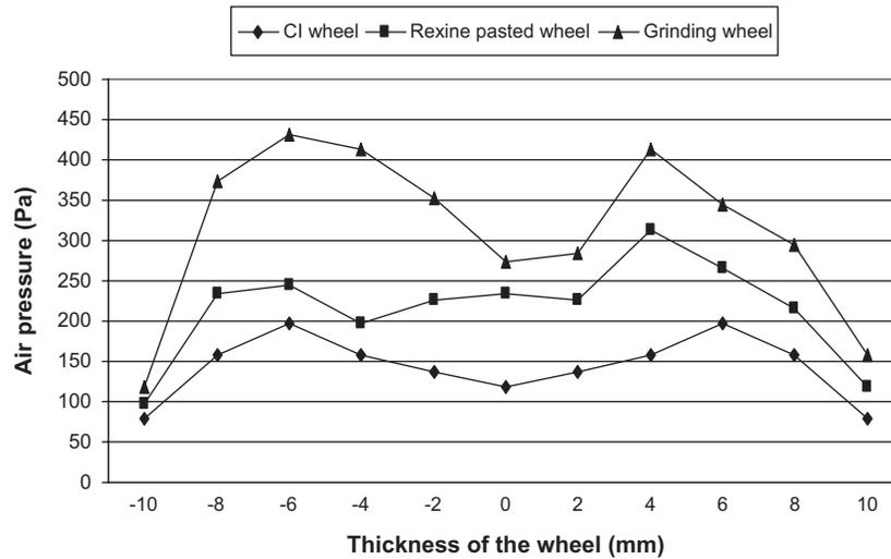
**Figure 11. Percent increase in pressure in grinding wheel than that of solid wheel along the thickness of the wheel.**
