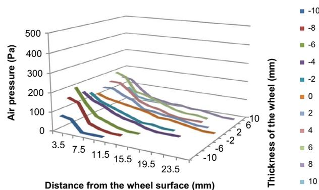
**Figure 9. Variation of air pressure in radially outward direction at a width wise location 4 mm from 0-0 position.**
