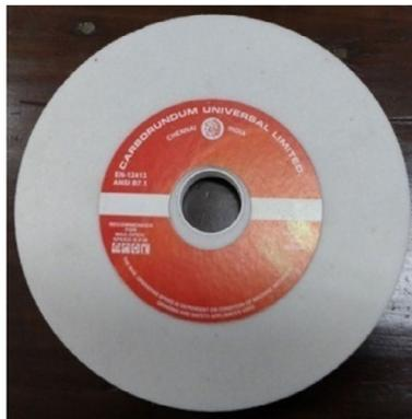
**Figure 3. Rexine cloth covered alumina wheel.**
