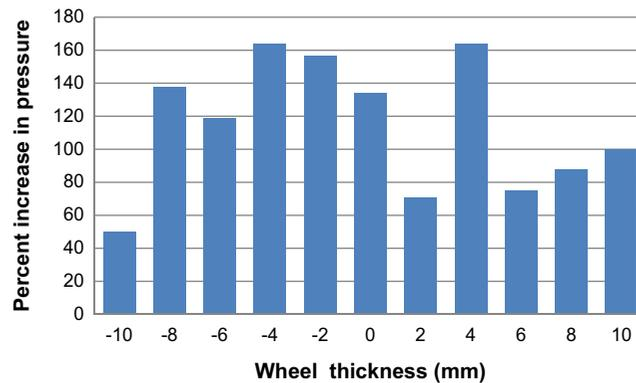
**Figure 12. Percent increase in pressure in rexine pasting than solid wheel along the thickness of wheel.**
