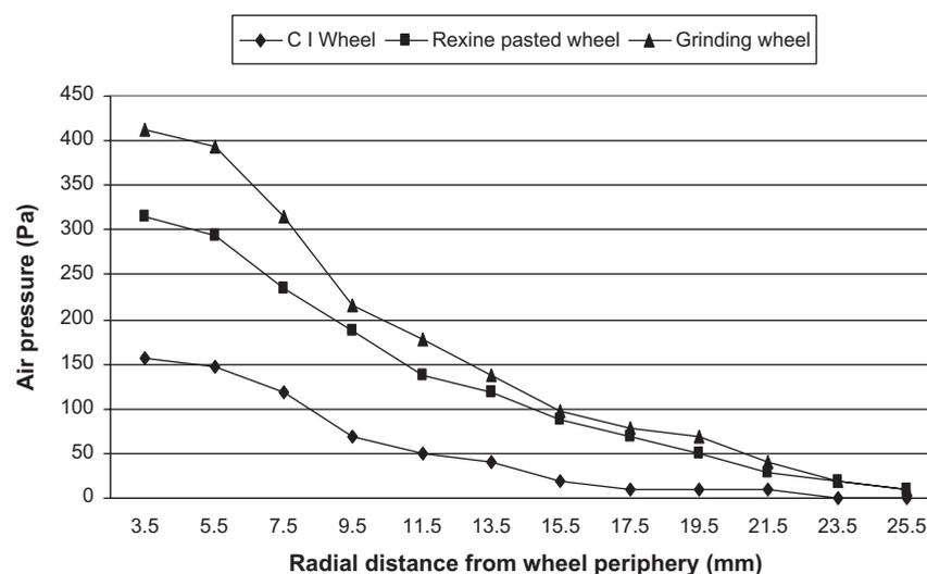
**Figure 10. Comparison of air pressure measured along the width of the rotating wheel at a fixed distance from periphery.**
