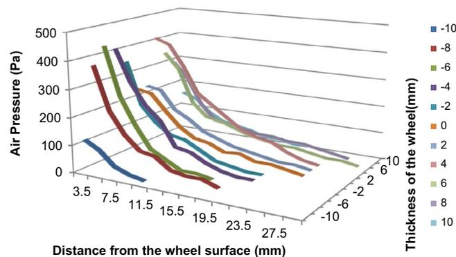
Figure 7. Variation of air pressure in radially outward direction and at various points along the thickness of rexine-pasted grinding wheel.
