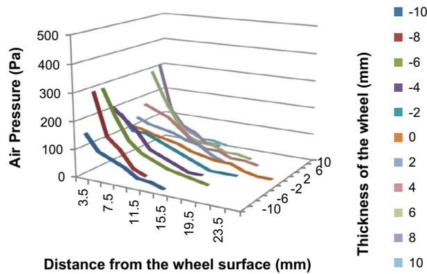
**Figure 14.** Variation of air pressure in radially outward direction and at various points along the thickness of rexine-pasted grinding wheel with scraper board.
