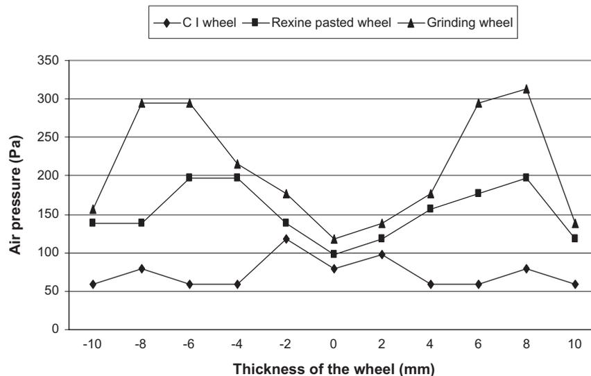
**Figure 18. Average percentage increase in pressure in different wheels with comparison to solid wheel.**
