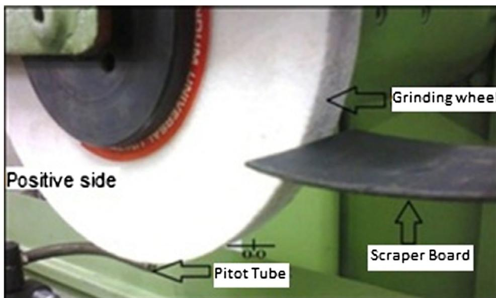
In another set of experiment, a PVC scraper board is used in intend to obstruct the air layer formed due to the rotation of wheel in static air. Arrangement of scraper board with wheel is shown in Figure 5. Conditions for experiments performed using grinding wheel are outlined in Table 2.
