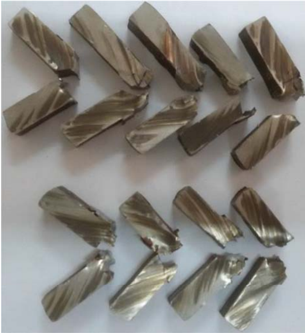
Fig. 7. Impact test samples after fracture
