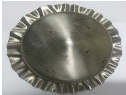
Figure 8: Component Formed by Conventional Deep Drawing
