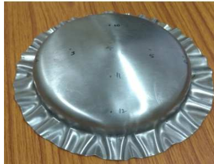
Figure 9: Component Formed by Rubber Assisted Deep Drawing
