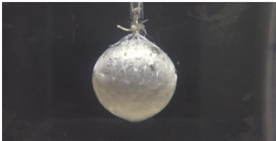
Figure 10. Air bubbles during melting of ice
