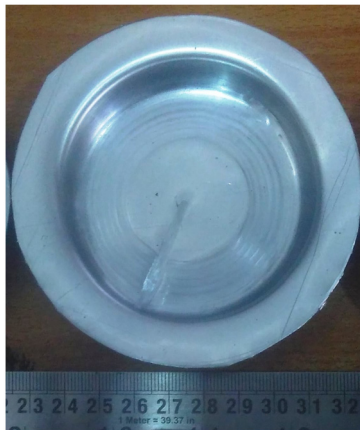
Fig. 8. Final product after implementation modified MSMS forming strategy.
