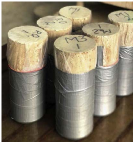
Fig. 2. Configuration for the rate of water absorption and coefficient of water absorption test.
