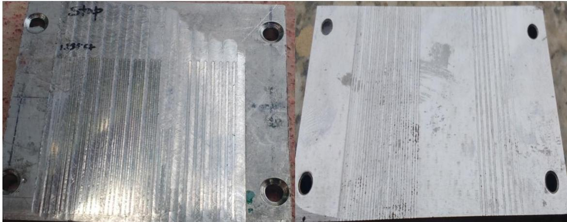
Figure 2. Specimens after micro-end milling experiments: (a) Titanium alloy; (b) Mild steel
