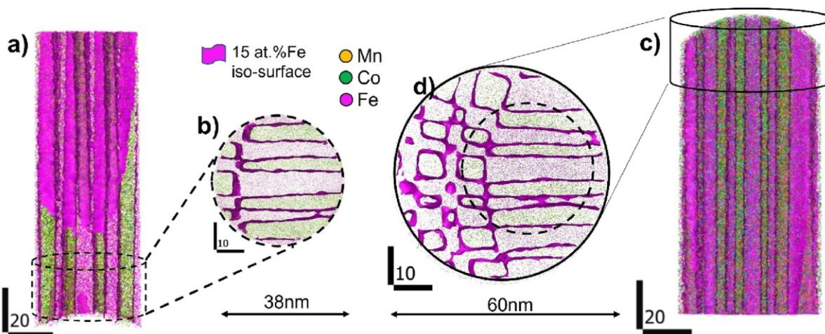
**Fig. 1.** a) Reconstructed volume of the spinel CoFeMnO mixed oxide acquired using a LEAP 6000 XR. The plate-like phase separation is evident in Figure 1b which is taken from the last 20nm of the data in Figure 1a. c) Reconstructed volume from the same tip acquired on an Invizo 6000. d) The radial FOV of Invizo is 1.6X larger than LEAP 6000 XR allowing the chessboard structure to be viewed in the left-hand side of the detector. The improvement in FOV translates to 2.5X in areal FOV.
