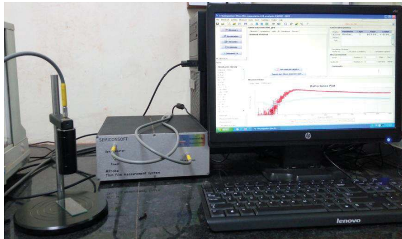
Figure 2.16: MProbe thickness measurement set up.
