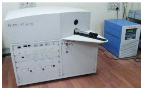
Figure 2.11: X-ray photoelectron spectroscopy setup (Amicus).
