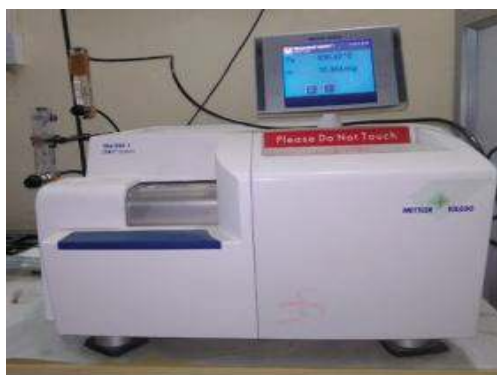
Figure 2.4: TGA-DSC set up.
