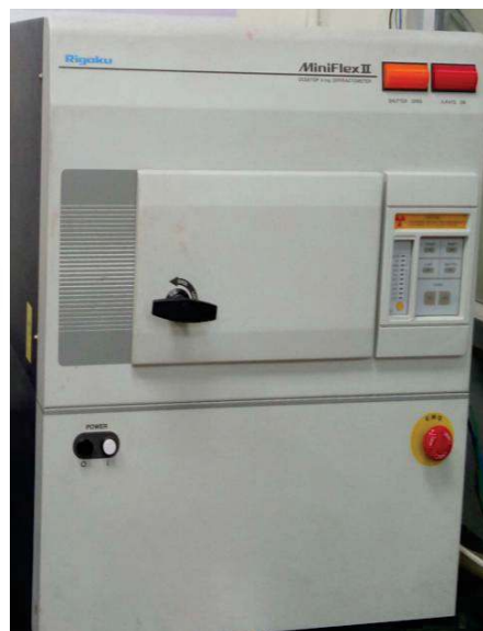
Figure 2.5 (a) Schematic diagram of X-ray diffraction (b) XRD set up.
