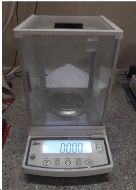
Figure 2. 1: Electronic balance for weight measurements of the powder materials.
