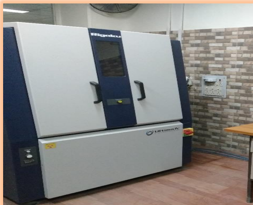
Figure 2. 6: X-ray powder diffraction (XRD) instrument.
