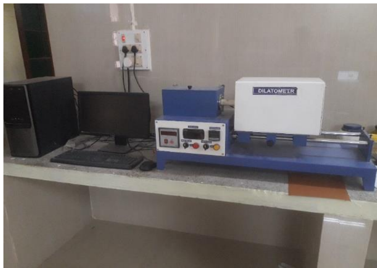
Figure 2. 12: Dilatometer used for measurement of thermal expansion of the sample.
