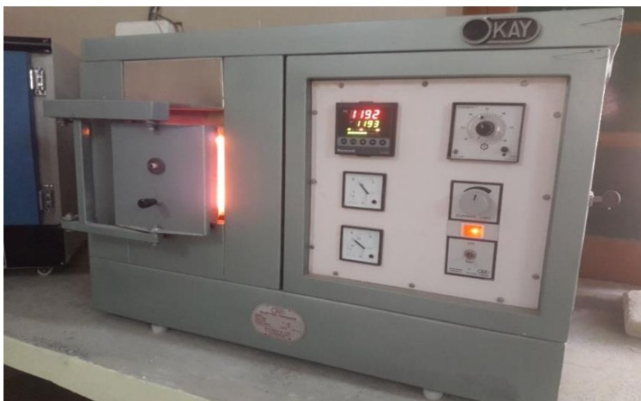
Figure 2. 5: Electric silicon carbide furnace.
