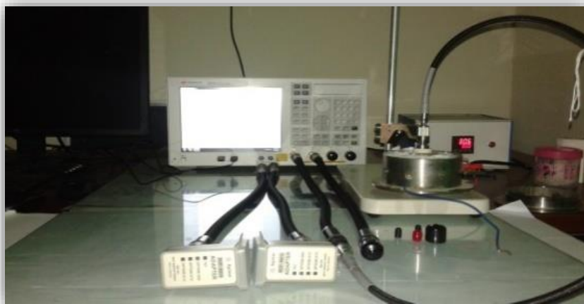
Figure 2. 15: An instrument vector network analyzer used for measuring dielectric constant and loss tangent at a microwave frequency (1-20 GHz).
