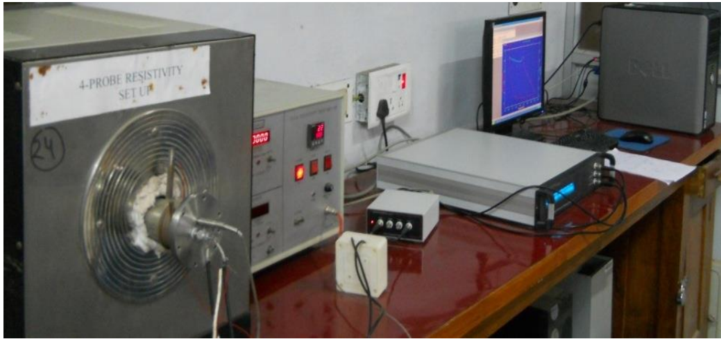
Figure 2. 14: Novo control Alpha-A Frequency Analyzer with the furnace and the required interfaces.
