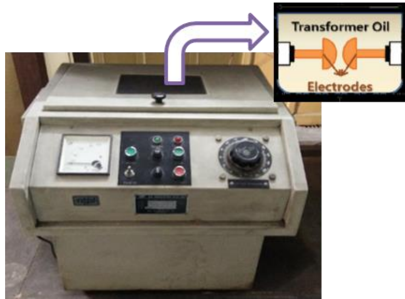
Figure 2. 13: Voltage breakdown insulation test (1 to 150 KV).
