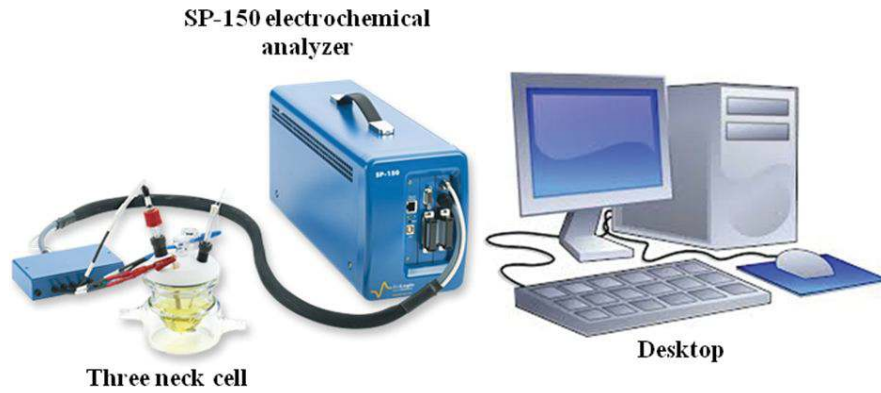
FIGURE 3.12: Schematic Layout of experiment setup used for corrosion test.
