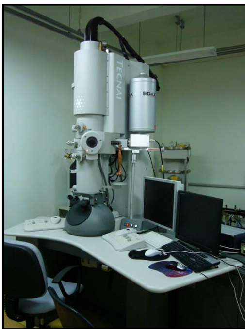
Fig.2.4. Transmission Electron Microscope (TEM, FEI TECANI G 2 20 TWIN, USA) used to determining particle structure.
