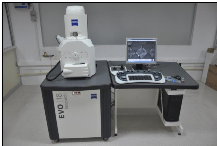
Fig.2.5. Scanning Electron Microscope (ZEISS, model EVO-18 Research) used for microstructure of the surface of the ceramics.
