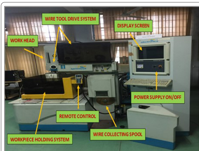
Figure 2: WEDM machine setup (Sprint cut 734).
