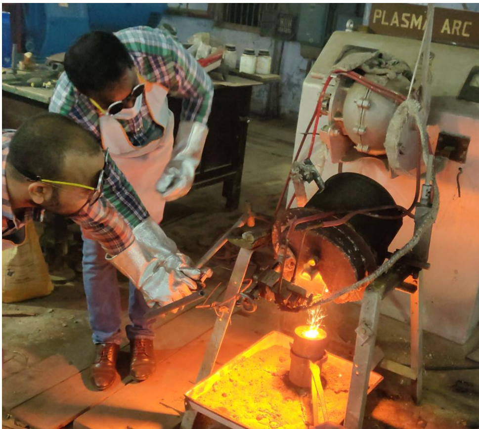
Figure 5.2 Tapping of the melt in a graphite crucible.
