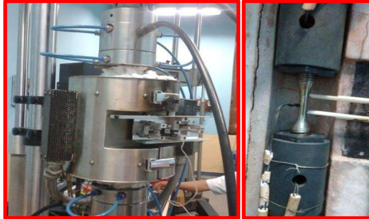
Fig. 2.5 (a) Machine set up for high temperature ratcheting fatigue experiments and (b) High temperature extensometer and thermocouples mounted on the sample.
