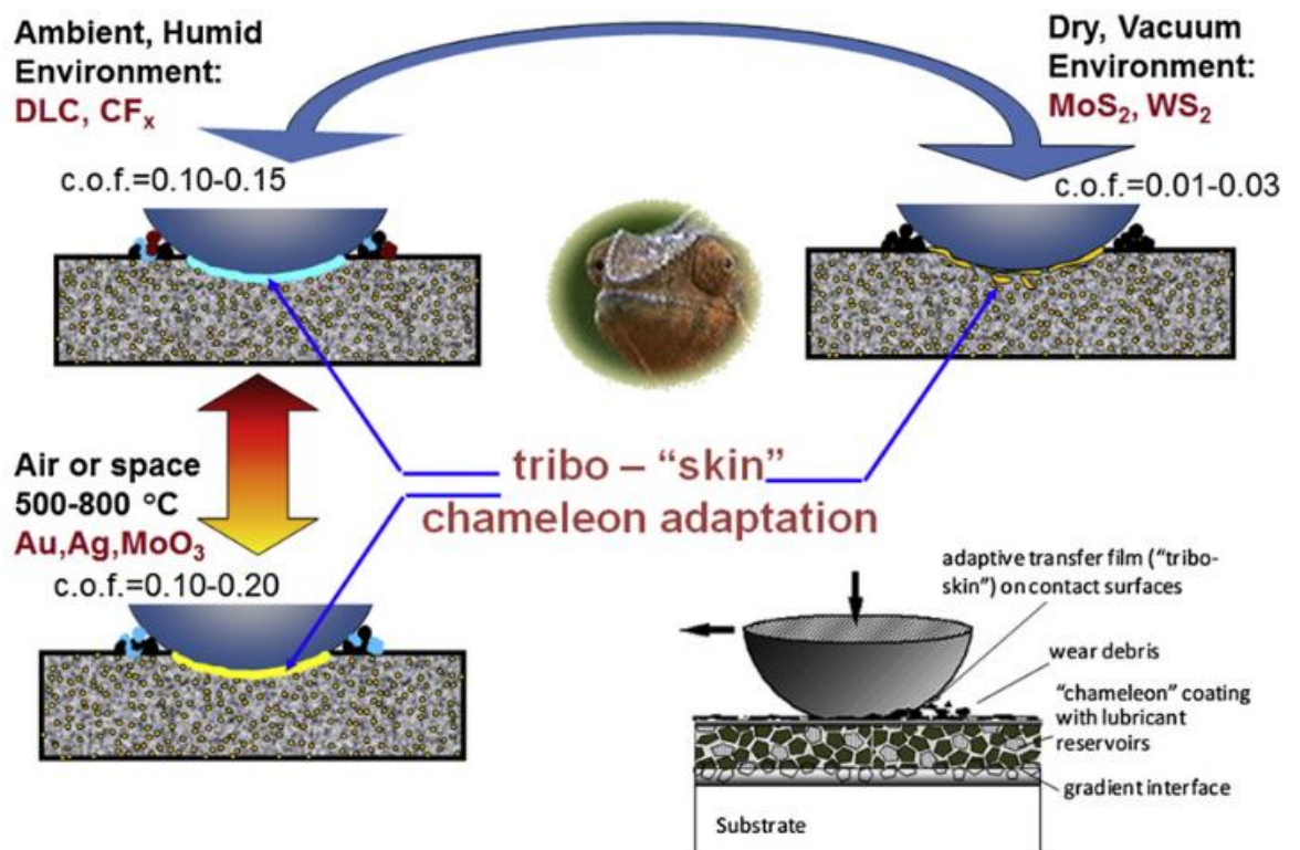
Figure 2.7. Schematic representation of chameleon adaptive coatings. Reprinted with permission from reference [126].
