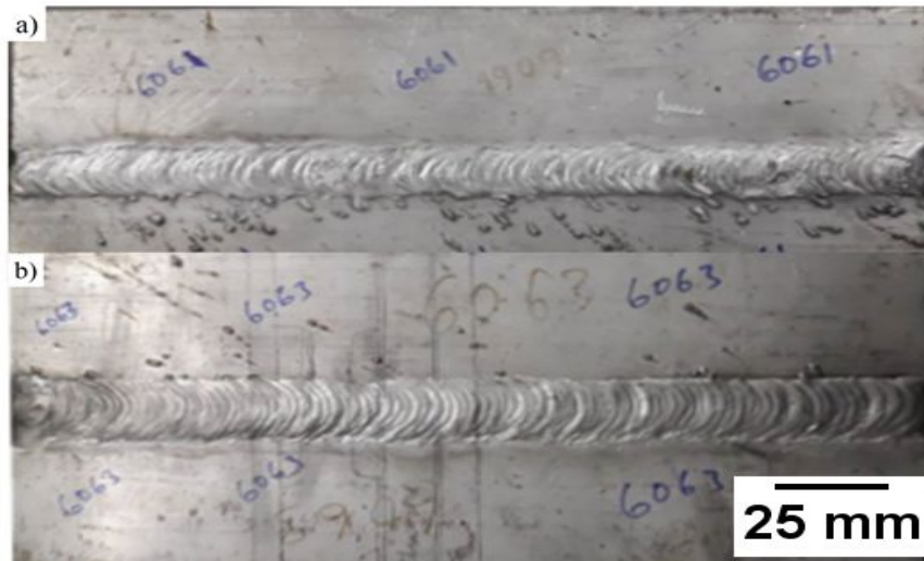
Figure 3.9: The Welded plates of a) A6061 and b) A6063
