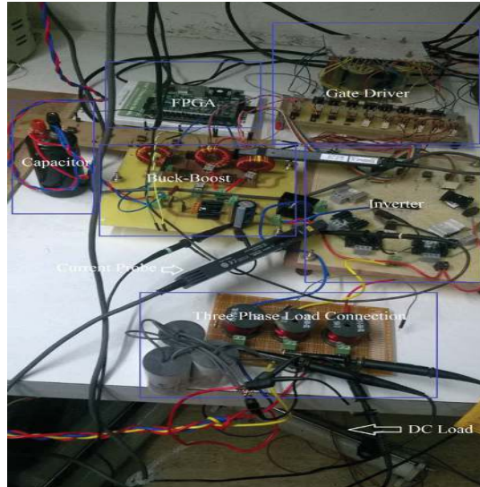
Figure 8.13: Experimental setup for MBBDHC
