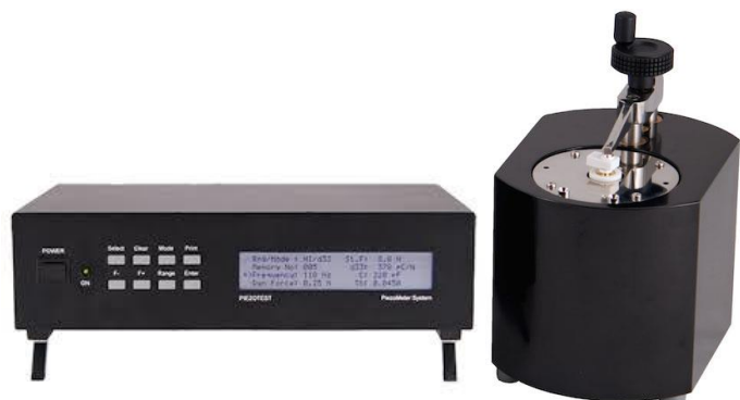
Fig 2.8 A typical d_{33} meter instrument
