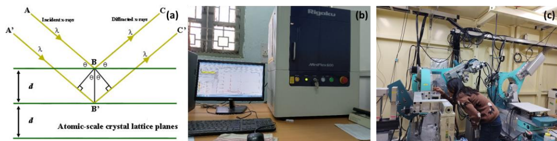
Fig 2.4 (a) Principle of Bragg's law for visualizing XRD, (b) Cu K_{\alpha 1} based laboratory XRD Rigaku Miniflex and (c) Synchrotron XRD measurement station hutch
