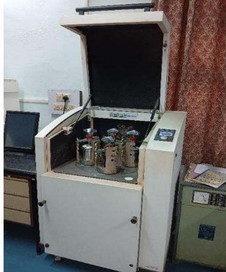
Fig 2.1 A typical Retsch PM400 MA high energy ball mill
