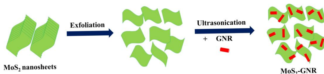
Figure 5.3 Schematic pathway for the synthesis of MoS 2 -GNR nanocomposite
