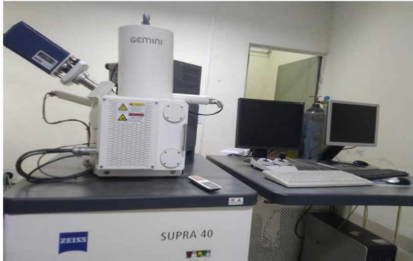
Figure 2.3: Image of Scanning electron microscope ZEISS SUPRA 40.
