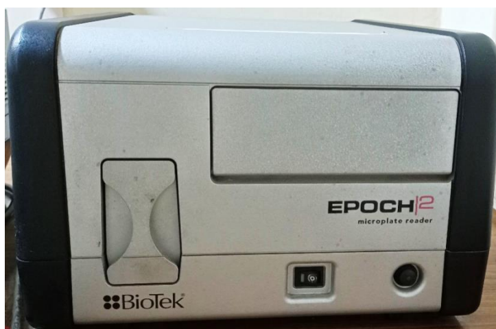
Figure 2.2 UV-Vis spectrometer (EPOCH microplate reader (Biotek, Courtesy IIT BHU))
