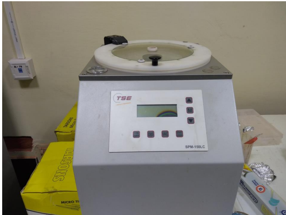
Figure 2. 2: Spin coater setup for thin film deposition.
