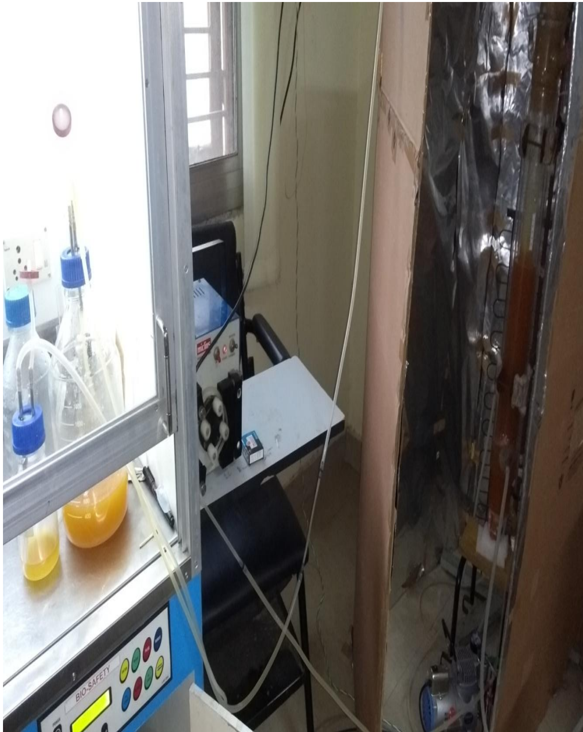
Fig 4.19 Fermentation set up of internal loop ALR
