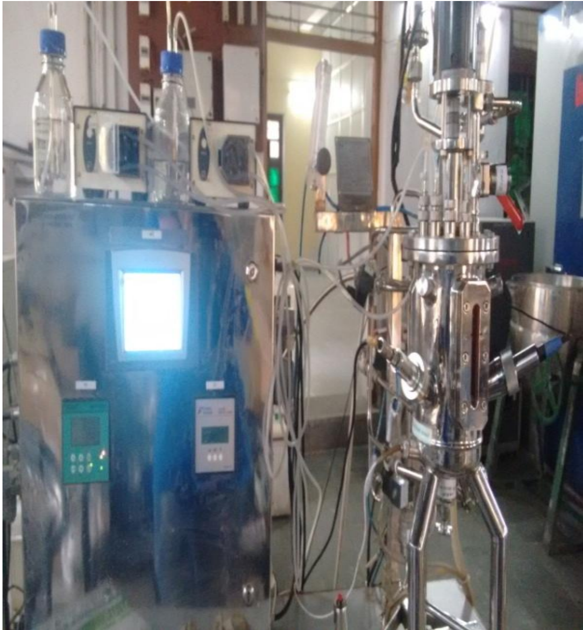
Fig 4.4 Production of rapamycin in 3L Stirred tank reactor (Scigenics, India)
