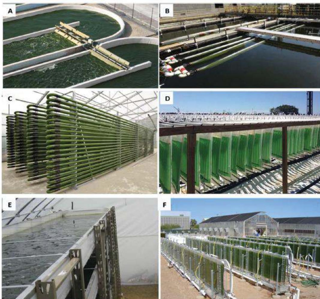
The above figures (A) to (F) shown the various reactor configuration for microalgal cultivation at (A) raceway pond (from Sapphire Inc, America); (B) Floting photobioreactor (from OMEGA system- ASA); (C) tubular bioreactor (Wolfsburg, Germany); (D) Plastic Bag bioreactor (from Algenol Inc, America); E) Multi-layer bioreactor (from center for biorefining, University of Minnesota; (F) Flat-panel Bioreactor (from Nanovoltaics technologies, America) [103]
