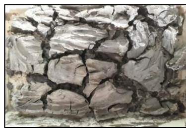
(a) In-site and laboratory dried Marine soil
