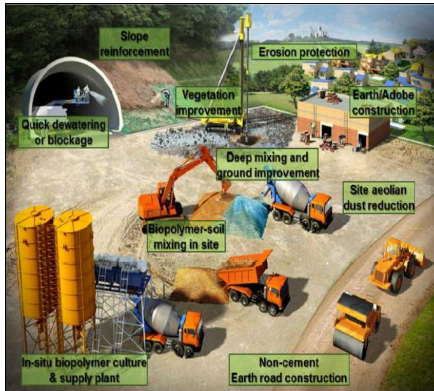
Figure 1.2 Biopolymer applications in geotechnical engineering practices [36]
