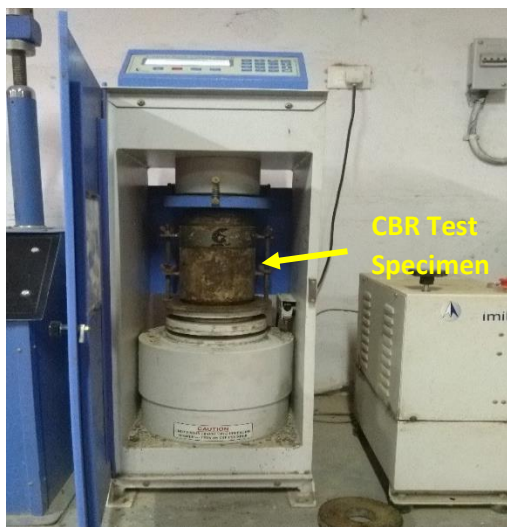
Figure 3.8 Static compaction of the specimen through a compression machine.
