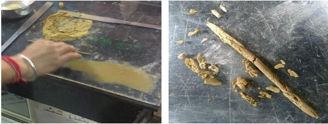
Figure 3.3 Plastic limit of soil mixtures.
