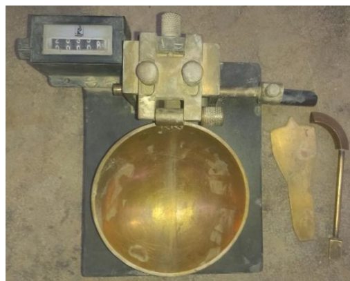
Figure 3.2 Casagrande apparatus for liquid limit.
