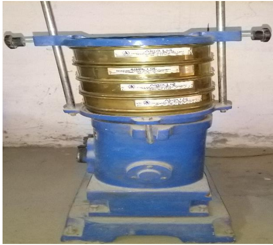
Figure 3.4 Mechanical sieve shaker for particle size gradation analysis.
