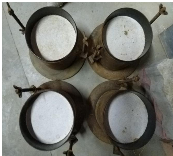
Figure 3.9 Laboratory prepared remolded CBR specimen.
