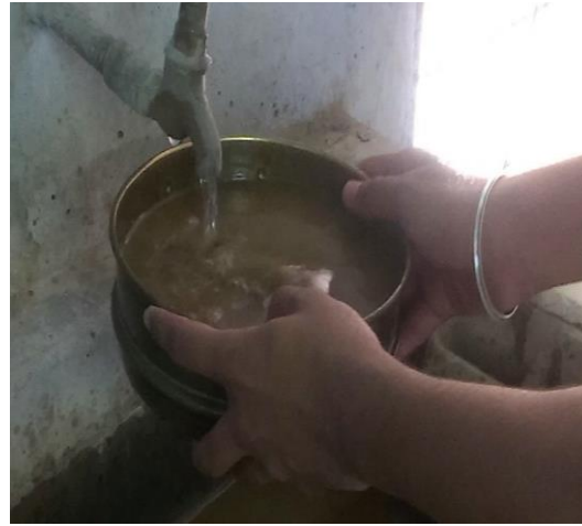
Figure 3.5 Wet sieve analysis through 0.075 mm sieve.
