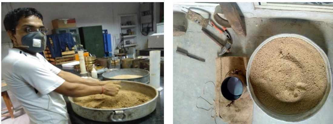
Figure 3.7 Preparation of materials for CBR specimen.
