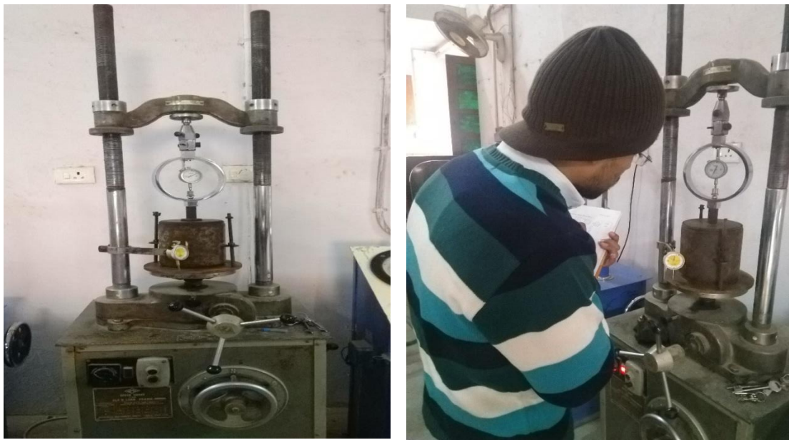
Figure 3.11 A complete test setup of CBR loading frame.
