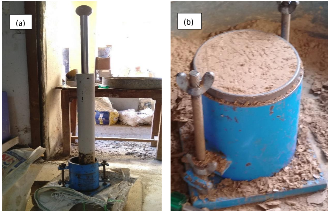
Figure 3.6 Modified Proctor compaction of soil samples.
