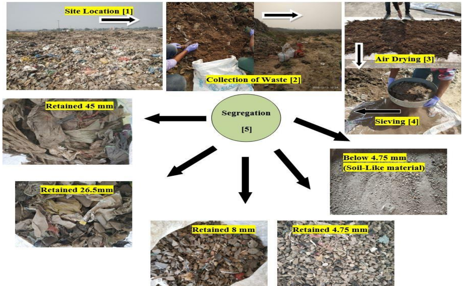
Figure 3.2 Cycle showing collection and segregation of MSW fine fractions
