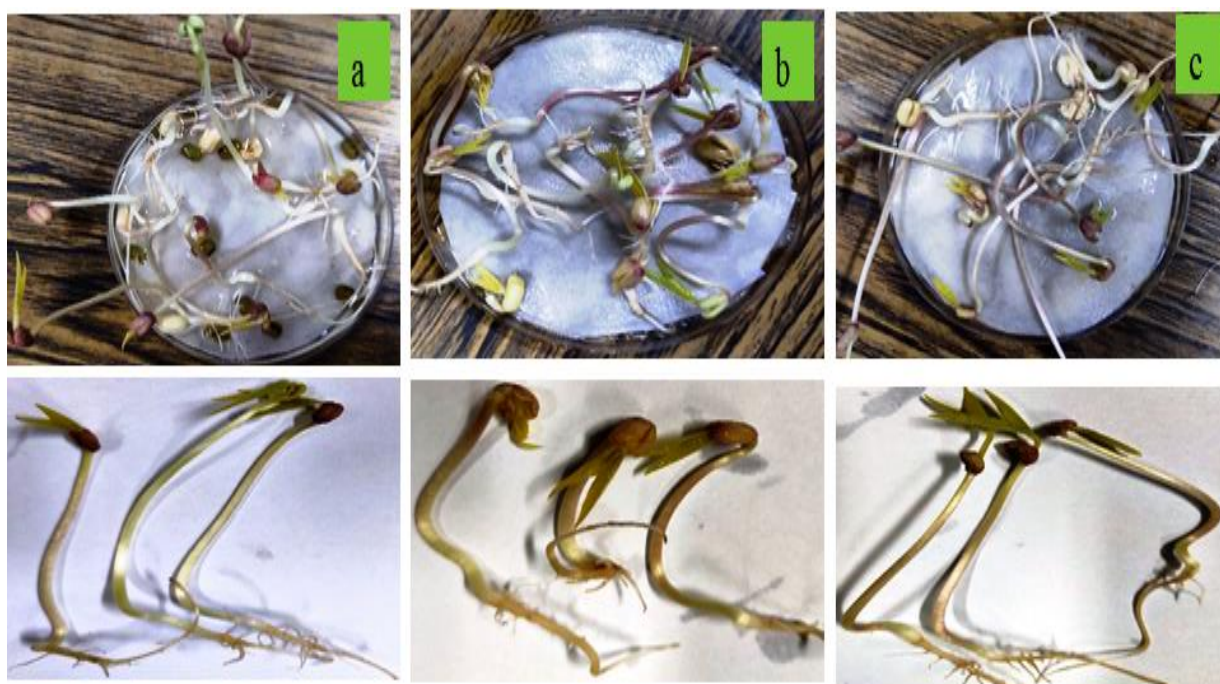
Figure 4.22. Images of Vigna radiata seeds germinated in (a) distilled water, (b) untreated wastewater, (c) treated wastewater (after 7.0 days).
