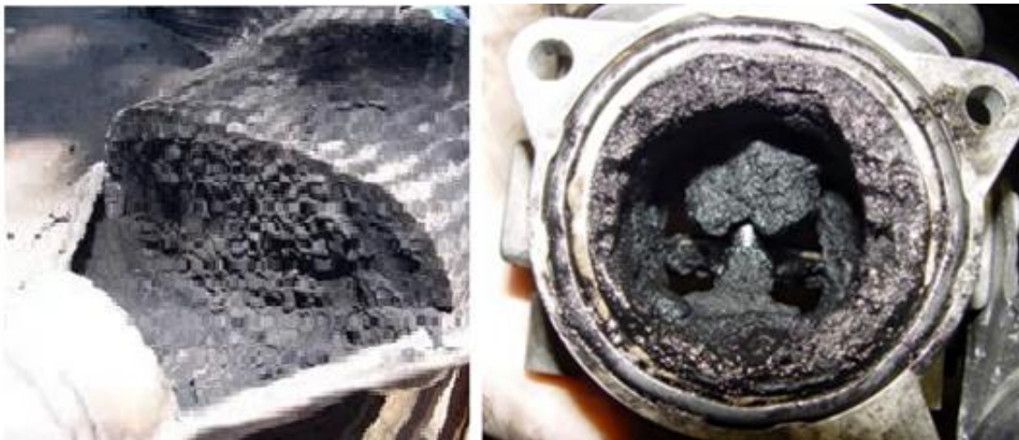
Figure 1.25 DPF damage due to high temperature
