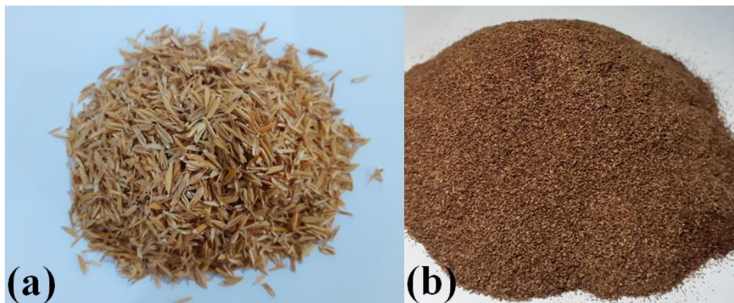
Fig. 4.4 (a) Throughly washed RH and (b) processed RH powder
