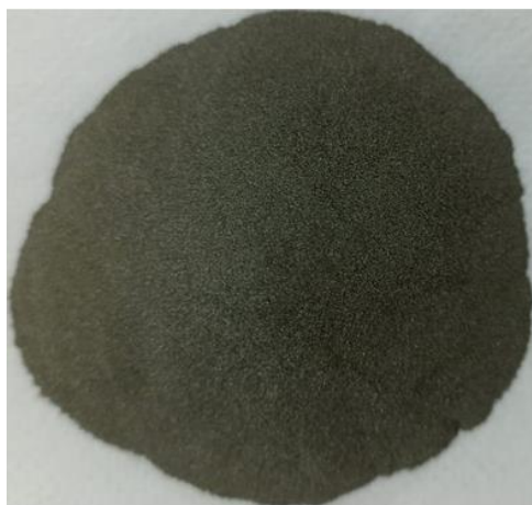
Fig. 4.3 Titanium (Ti) metal powder of 100 mesh particle size
