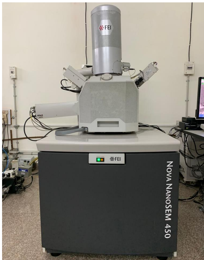
Fig. 4.7 Scanning Electron machine setup
