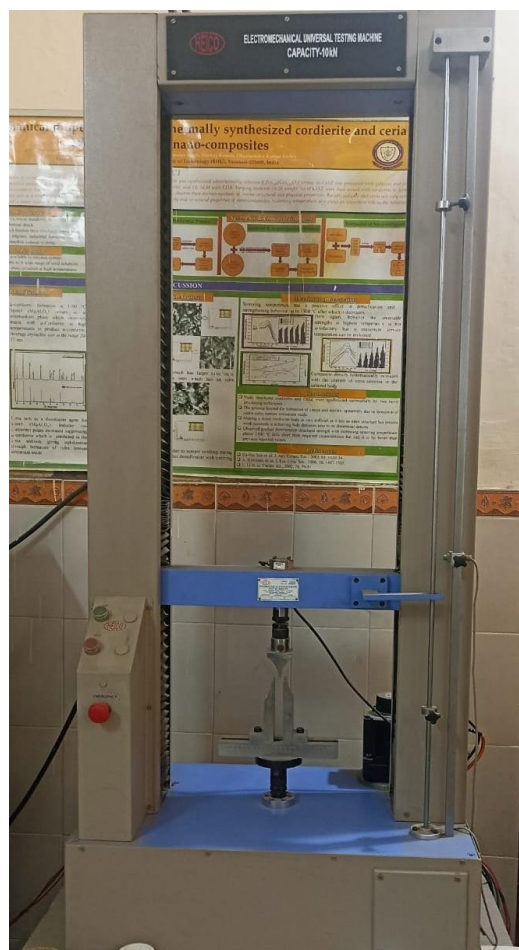
Fig. 4.10 UTM machine for measurement of compressive strength
