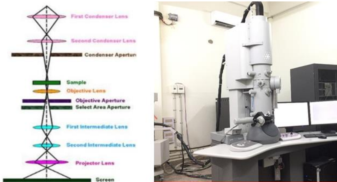
Fig. 4.9 Schematic representation of principle of Transmission electron microscopy (TEM) and Photograph of TEM
