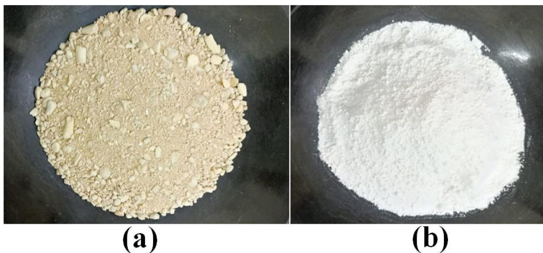
Fig. 4.5 (a) unsintered bone powder and (b) sintered bone powder
