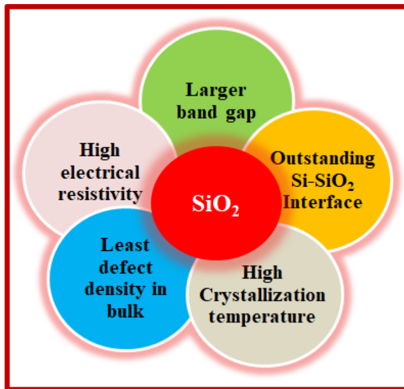
Figure 1.6: Benchmarks to select the high-k dielectric for a thin film transistor.
