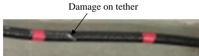
Figure 9.1: Damaged tether part towards the balloon end
