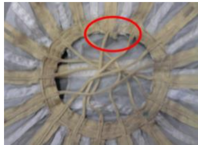
Figure 6.7: Vent-lines broken from vent band
