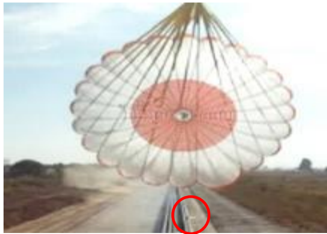
Figure 6.9: Suspension-lines broken near skirt band
