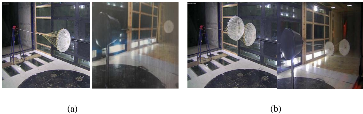
Figure 5.14: Wind tunnel test setup (a) single parachute with and without FB (b) a cluster of two parachutes with and without FB
