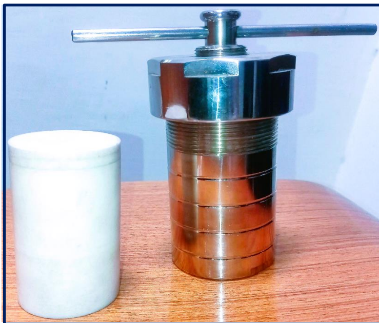
Figure 2.2 Photograph of the used hydrothermal cell.
