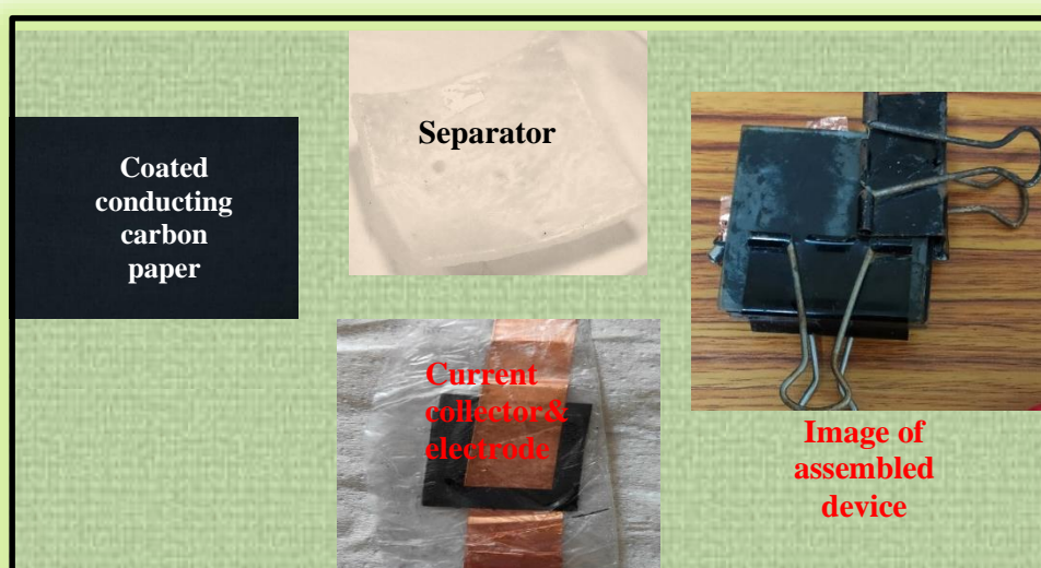
Figure 2.17 Photographs of components of solid-state supercapacitor device.
