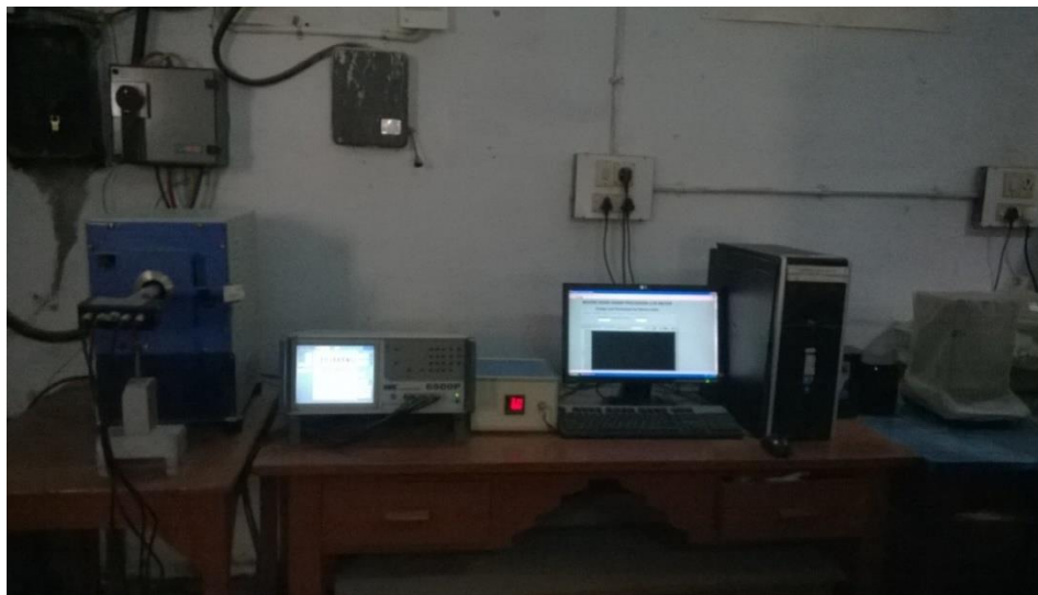
Figure 2.8 Computer-controlled LCR meter Set-up (Wayne Kerr 6500 P, U.K.)
