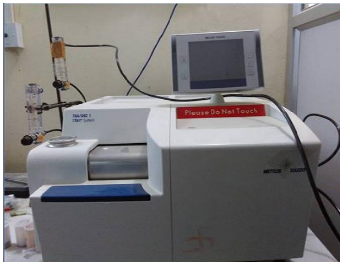
Figure 2.2 Experimental set-up of TG/DSC (Mettler Toledo, Germany)
