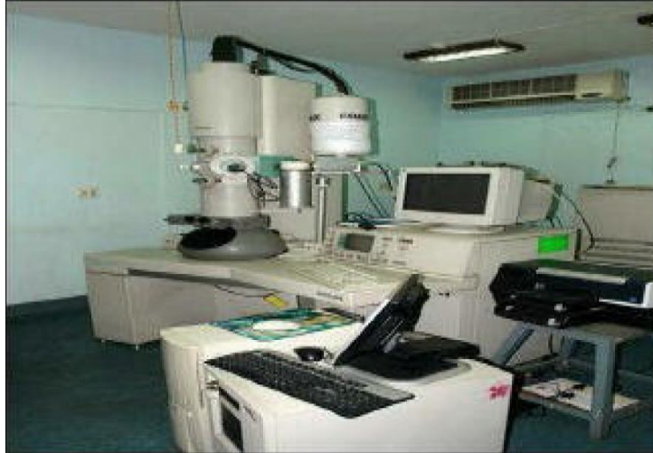
Figure 2.6 Experimental set-up of Transmission Electron Microscopy (TEM)
