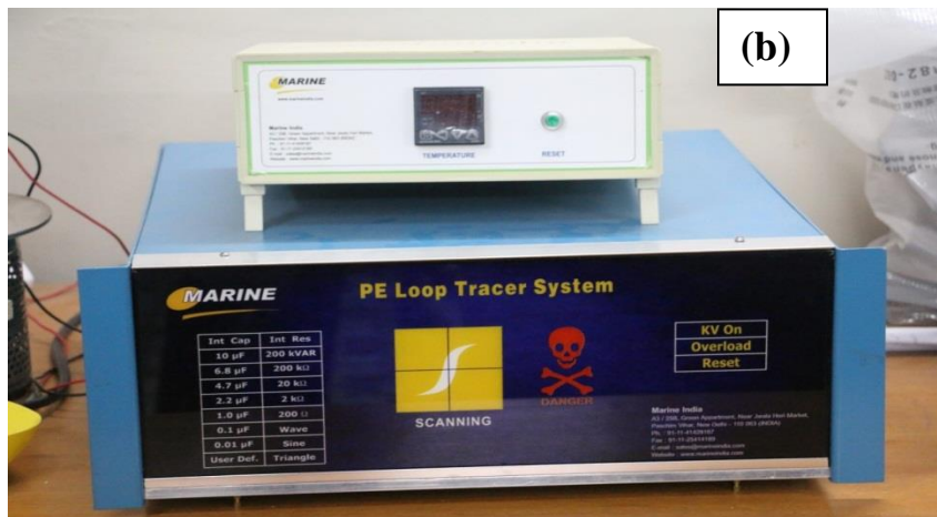
Figure 2.9 (a) Modified Sawyer-Tower Circuit for P-E measurements for bulk samples (b) P-E loop tracer setup (Marine, India)
