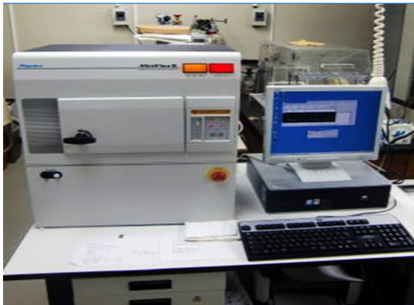
Figure 2.3 X-ray diffraction pattern (XRD) set-up ( Rigaku Miniflex II, Japan)
