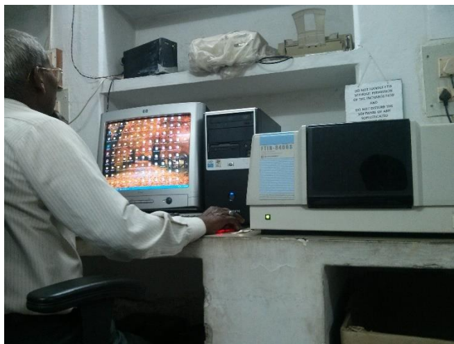
Figure 2.4 Experimental set-up FTIR spectrophotometer FTIR- 8400S, Shimadzu
