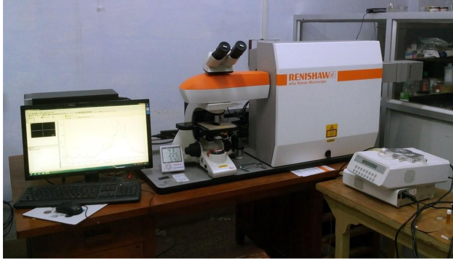
Figure 2.5 Experimental set-up of Raman spectrometer
