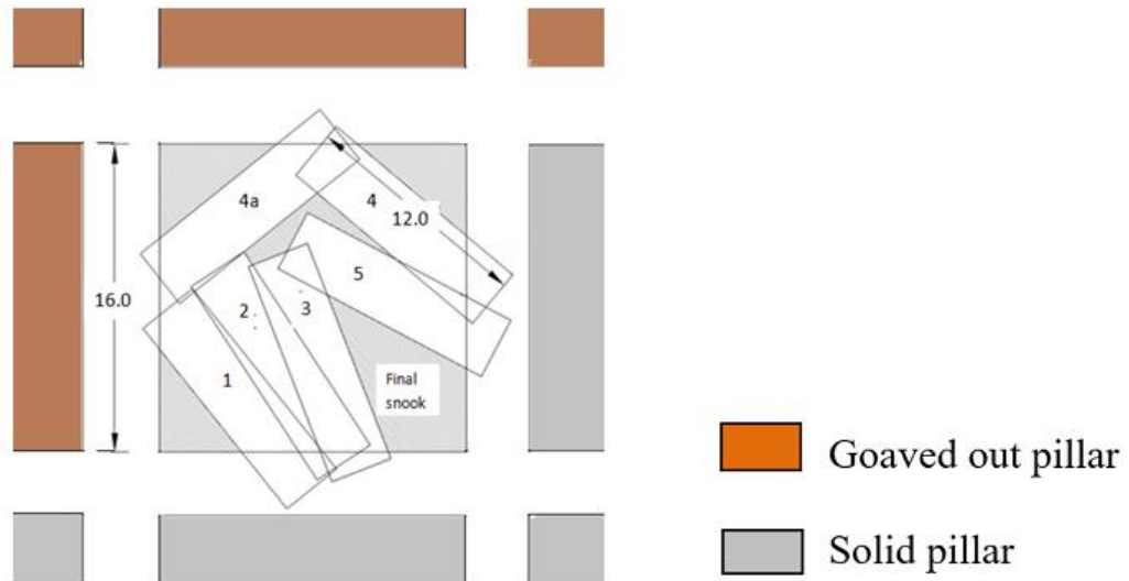
Fig.2.5. Modified Navid pattern of pillar extraction
