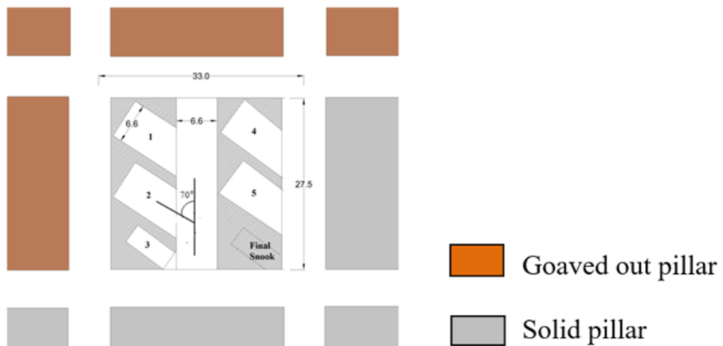
Fig.2.7. Split and fender pattern of pillar extraction
