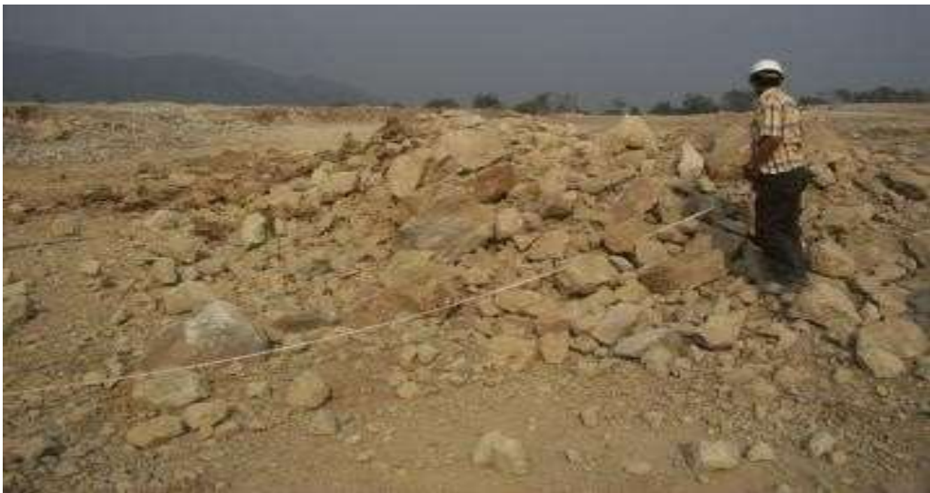
Figure 3.7: Post-blasting muck profile in Quarry ‘A’
