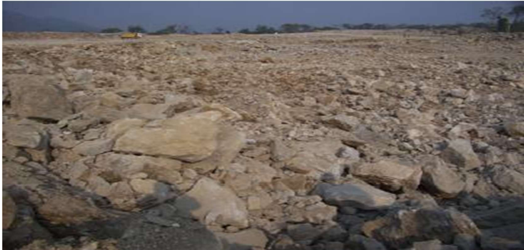
Figure 3.13: Post-blasting muck profile in Quarry ‘B’
