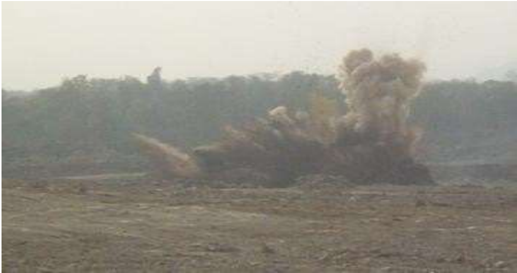
Figure 3.6: Blasting operation in Quarry ‘A’
