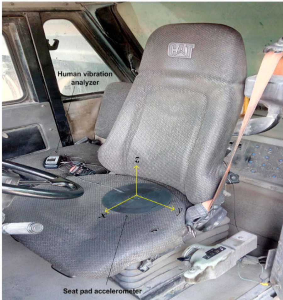
Figure 3.3 Positioning of seatpad accelerometer on dumper operator's seat
