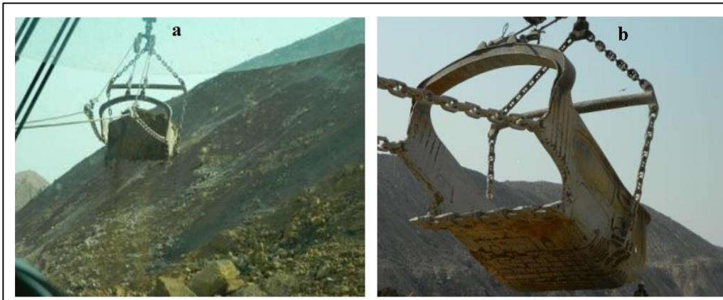
Figure 3.12 (a) loading and (b) unloading segment of a dragline cycle
