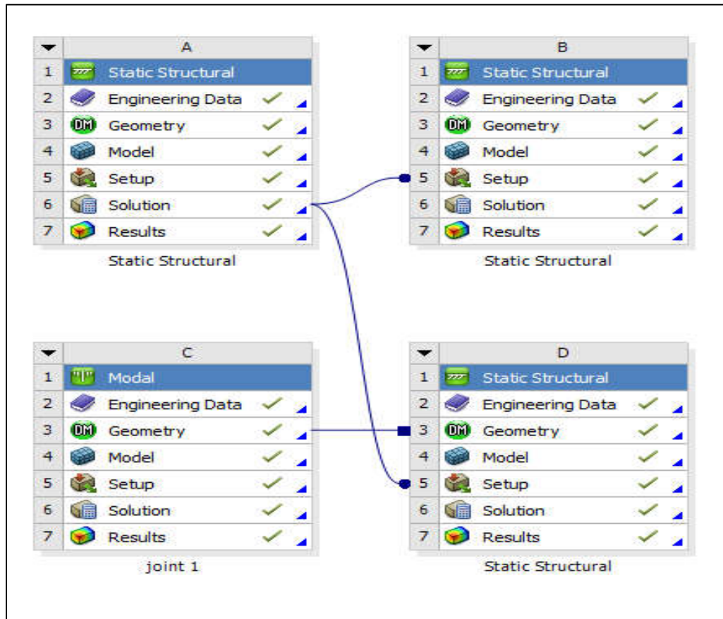
Figure 3.8 Solution procedures in ANSYS for a critical location in a global beam model
