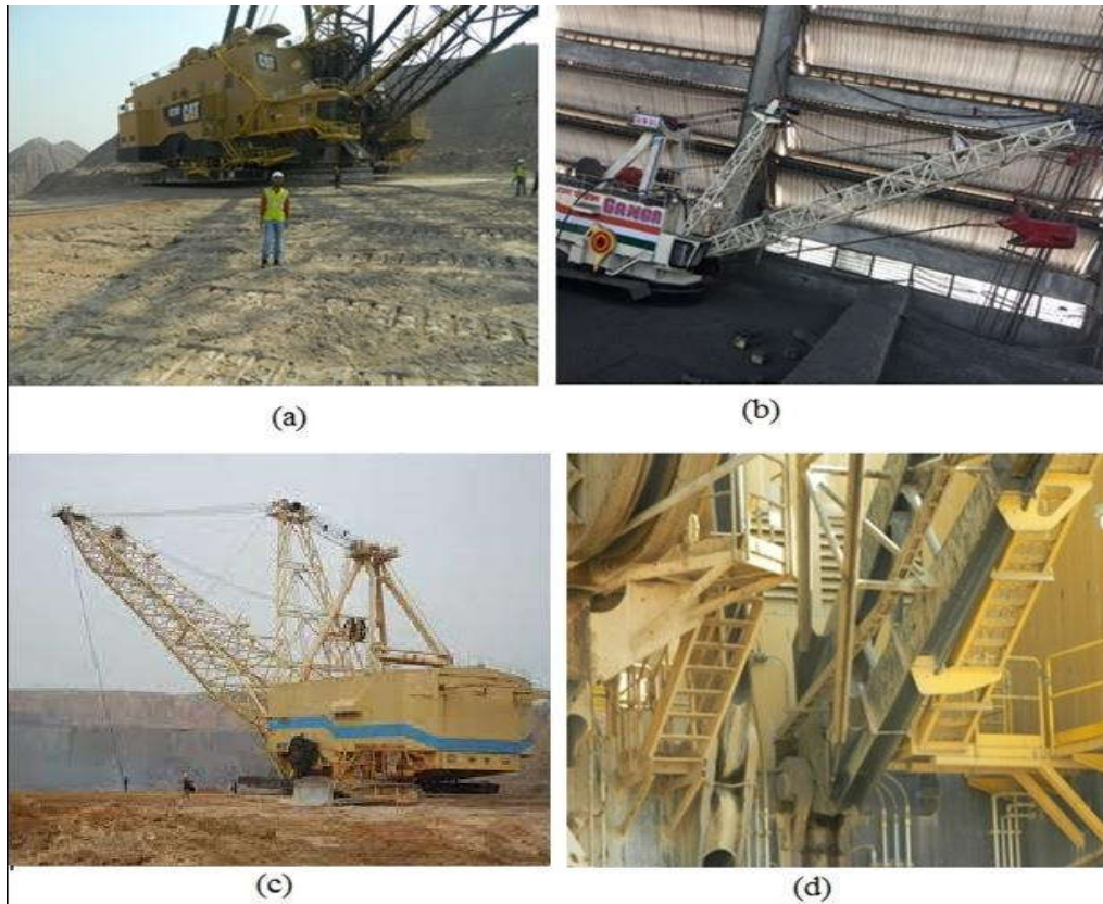
Figure 3.2 (a-d) Images from field visits. (a) Dragline model 8200 in SASAN coal mine (b) Ganga dragline model in NCL (c) 24/96 dragline model in NCL and (d) Zoom view of boom foot of the dragline
