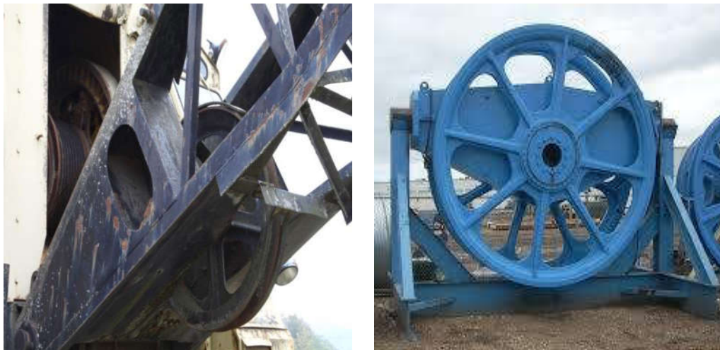
Figure 1.5 Boom foot and Boom point sheave of a dragline (Dragline Dictionary Edition, 2014)
