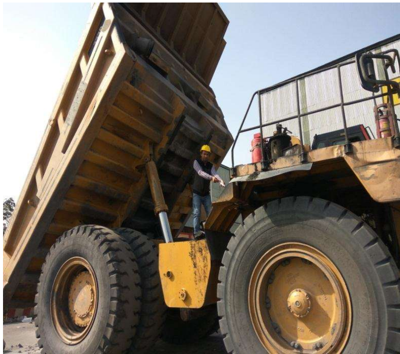
Figure 4.3 CO 2 measurement of dump truck by UNIPHOS gas detector tube and pump
