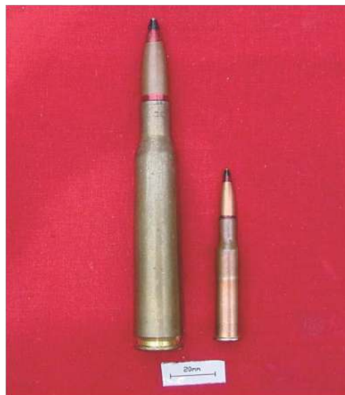
Fig 2.8: Different calibre projectiles used for ballistic experiments (Jena et al., 2016).
